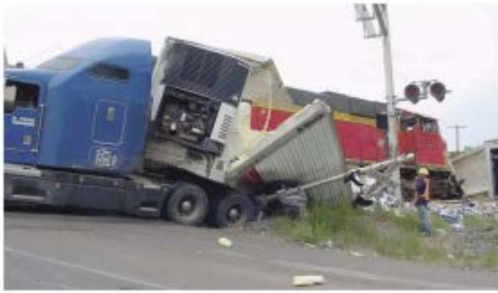
Figure 2.10 Aftermath of a hump crossing collision (Operation Lifesaver, 2015).
