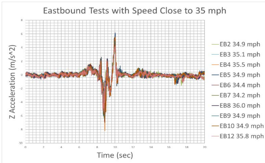
Figure 4.7 Eastbound tests with speed close to 35 mph.
